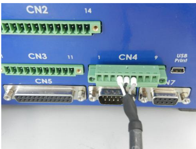
View connector CN4 - EDU 2AE/TOP unit
