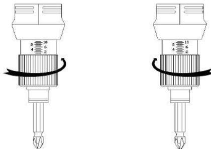
After each adjustment, it is possible to lock the nut with the clutch cover (sold separately). To place properly this cover, you must remove the stopper ring #2, unscrew the adjusting nut #3, unscrew and remove the front ring #1 and replace it with the clutch cover #35.
