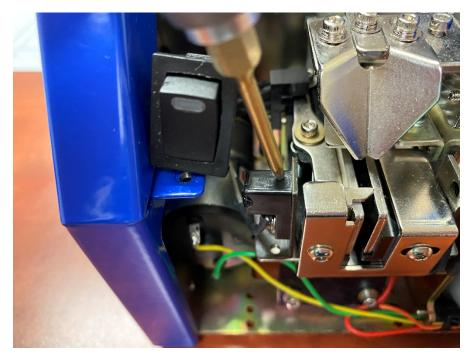
The sensors should be in matching positions on both side of the rail and aligned with the front portion of the rail where a screw rests after being fed.
